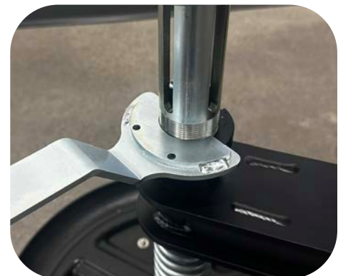
Beam And Outrigger Quick Change Cylinders
