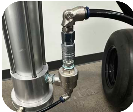
Cylinder Air Hose Quick Attachment
