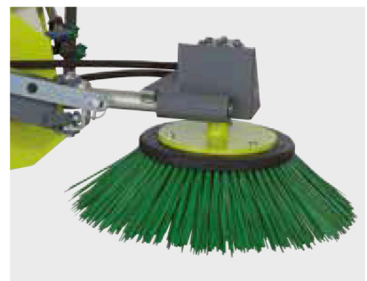
Hydraulic driven side brush in PPL
