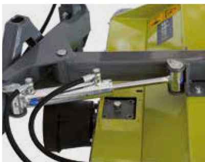
Hydraulic turn angle 250 left/right
