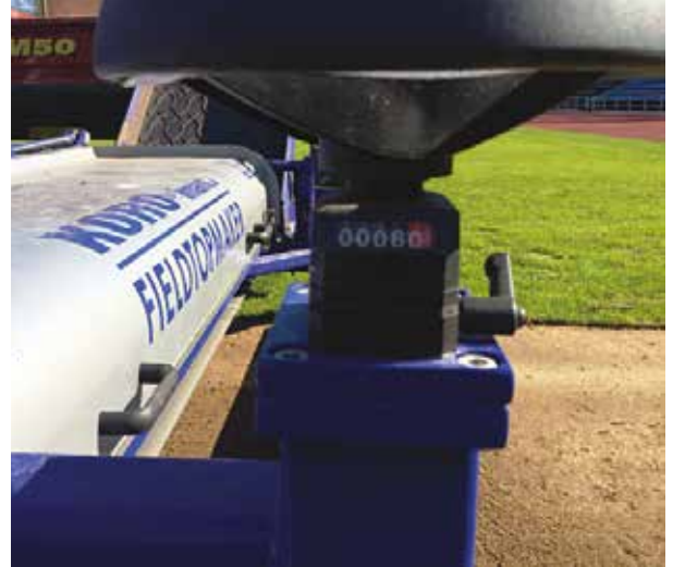
Depth setting is accurate to 0.1mm, via a digital display read out
