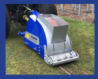
What is it? Secondary drainage tool which attaches to the RootPruner\* to allow sand slits.
