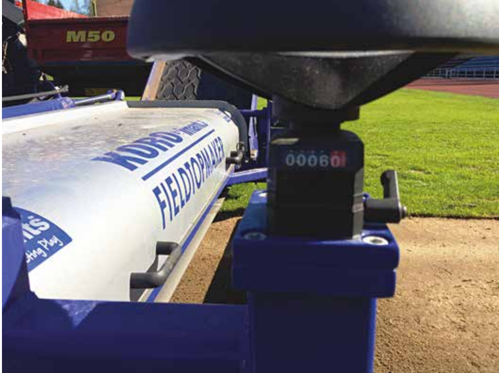
Depth setting is accurate to 0.1mm, via a digital display read out
