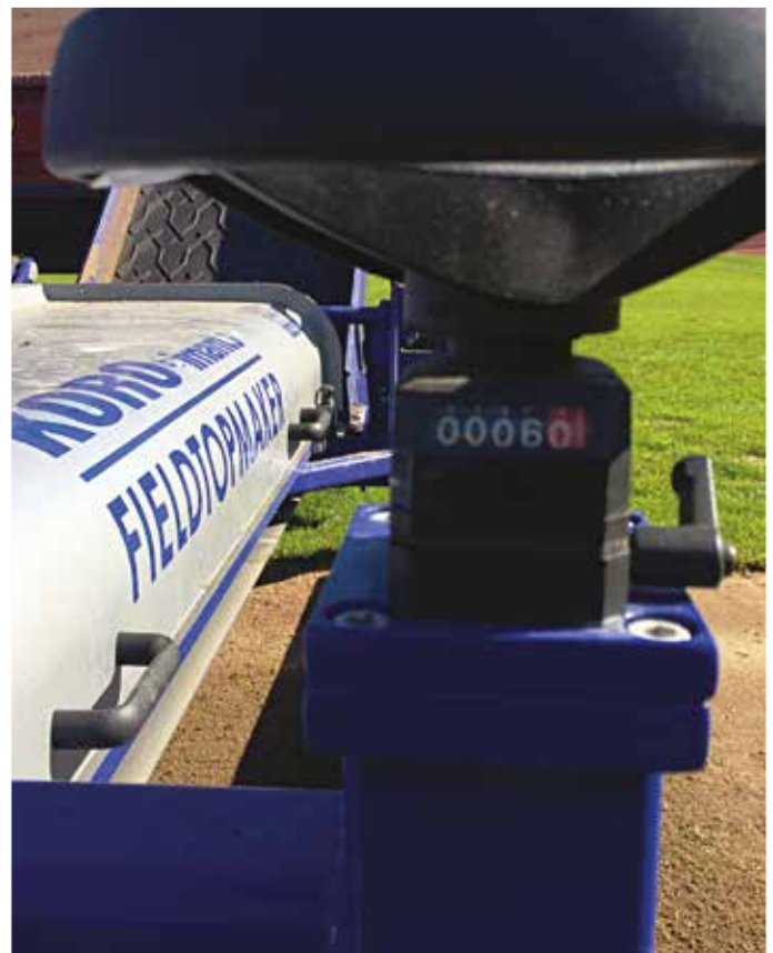
Depth setting is accurate to 0.1mm, via a digital display read out
