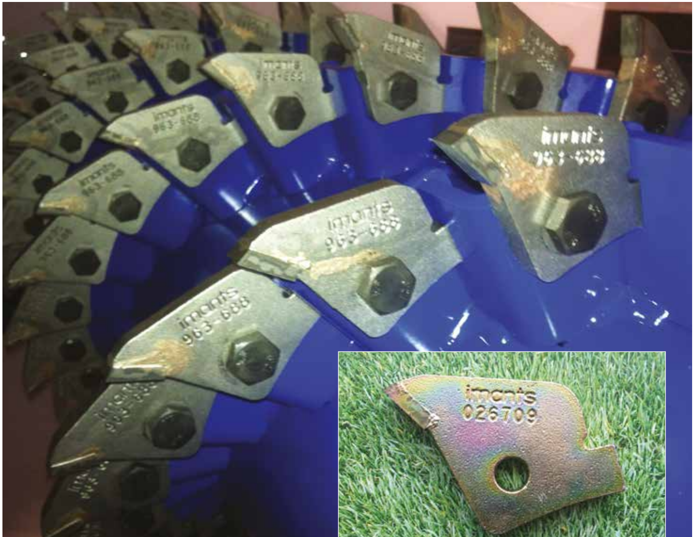
3/8" (10mm) tungsten tipped blades in 4 spiral Universe ® rotor configuration
