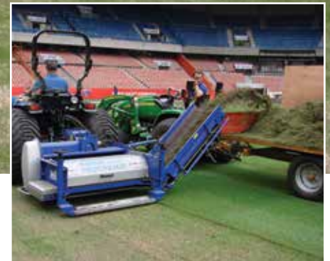
Lee Morgado and Simon Gumbrell carrying out the renovation using the Koro FTM.
